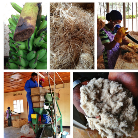
Figure 6. How SHE LaunchPads’ raw material is produced by banana fiber processing [9].
