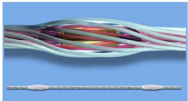
Figure 2. Electro-active polymer yarn with embedded actuator-sensor pair[9]
